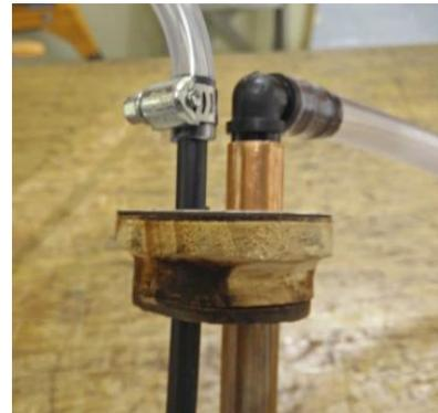
If used for heating water or other liquid, a continuous flow can be achieved by creating a stopper with two tubes for inflow and outflow.
